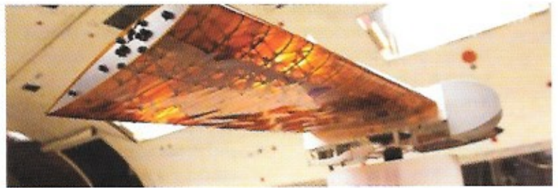
Bottom of page: The wing is constructed from building-block units made of advanced carbon fibre composite materials. (Photo: NASA/Kenneth Cheung)
