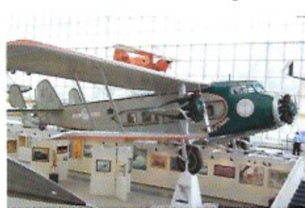
*The Model 80A trimotor biplane was to be the last word in luxurious air transportation. The 12-passenger transport had such features as forced-air ventilation, heat, and individual reading lamps. (Henry M. Holden)*
