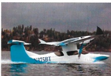
Left: The skis and the tri-hull have been tested at full scale on Lake Coeur d'Alene, validating performance and safety of the system. (Photo: Mike Kincaid)
