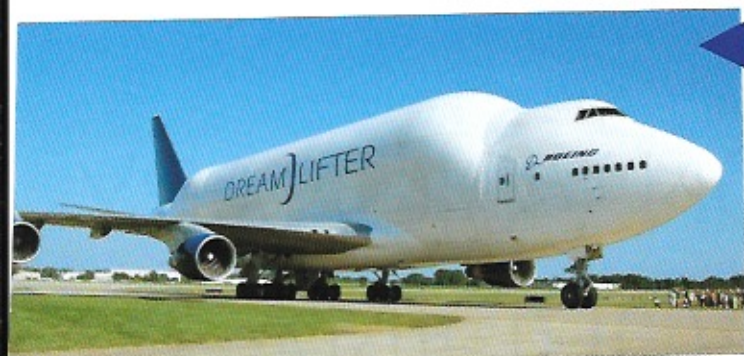
This aircraft is a specially modified 747-400 that transports the large composite structures, including huge fuselage sections of the 787 Dreamliner. The massive cargo is loaded and unloaded from a hinged rear fuselage. The last of the series of four was delivered Feb. 16, 2010. (Photo: Henry M. Holden)
