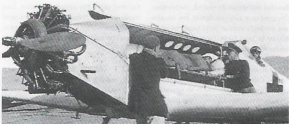
Below: In Dassault's MB 81, the patient was tucked away in a compartment between the pilot and the engine, where the pilot could keep an eye on his charge. (Dassault Aviation photos.)
