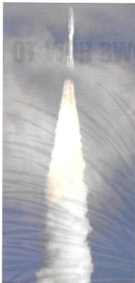
To get the kick needed to reach Jupiter and the outer solar system, New Horizons relied on a Star 48B solid-fuel motor that accelerated the small spacecraft to a departure velocity of some 10 miles per second, on course for a fly-by of Jupiter in late February 2007.
