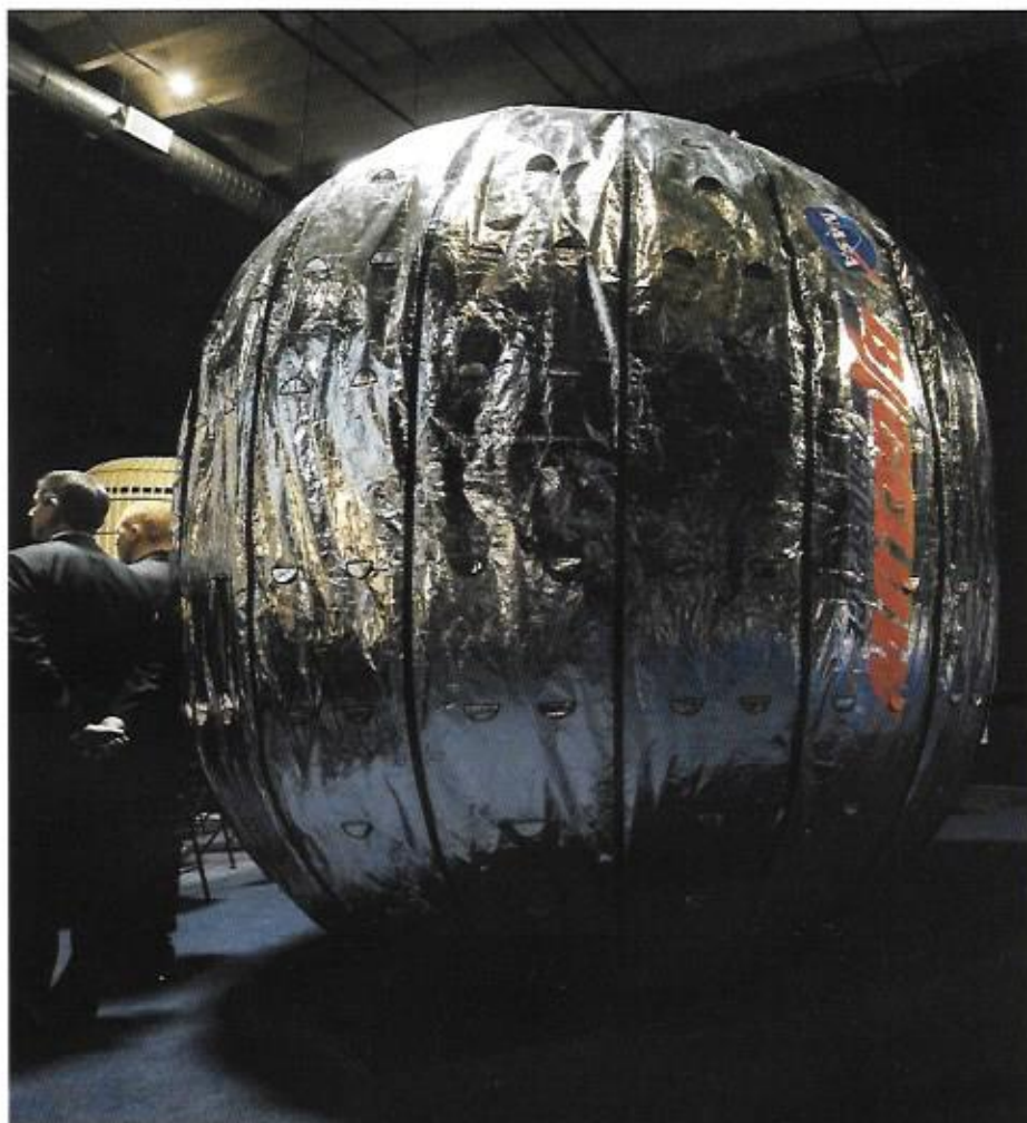
Top: BEAM can house four to six people in an approximate 6.7-metre long habitat. It will have a usable volume of 330 m 3 . The pressurised usable volume of a 20 ton B330 is 330 m 3 , compared with the 106 m 3 of the 15-ton ISS Destiny module, offering 210% more habitable space with an increase of only 33% in mass. Above: The Bigelow Expandable Activity Module (BEAM) is seen during a media briefing where NASA and Bigelow Aerospace announced that BEAM would join the International Space Station to test expandable space habitat technology. (Images: Bigelow Aerospace)
